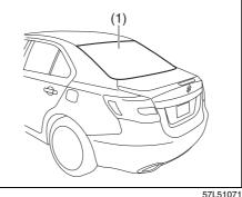
The radio antenna (1) wire is printed inside the rear window.
